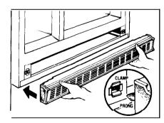
To replace base grille, align prongs on back of grille with clamps in cabinet and push forward until grille snaps into place.
